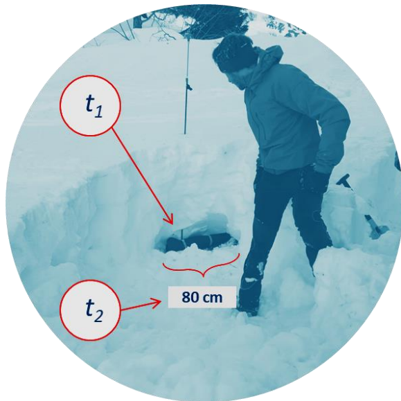
Figure 2: The measured parameters t_1 at probe tip reaching and t_2 at pit enlargement up to a constant dimension gauged with a dummy body.
